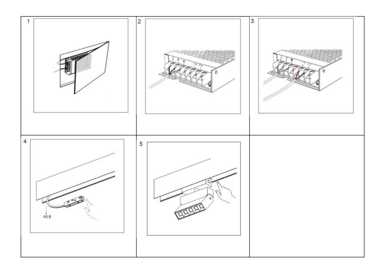
10.4 Connecting power supply to magnetic surface-mounted/suspended track using recessed power supply
