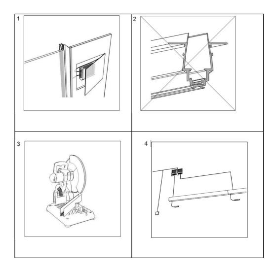
5. The power input can be installed in any section of the track, guided by rule, that one power input fee'ds no more than 20 meters of the track.
