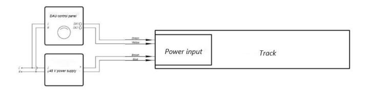
Attention! TRXO34DR4-100 / TRXO34DR4- 200 recessed power supplies cannot be used to connect DALI luminaire, since these power supplies do not have additional contacts for connecting the digital DALI protocol. To connect the digital DALI protocol, use TRAO04DR remote power supplies with power input.
