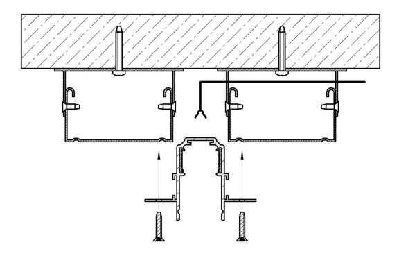
8. Install the plasterboard close to the track walls and secure it with screws. Bond a layer of fiberglass mesh. Cover the plasterboard with putty on the same level as the track walls.
